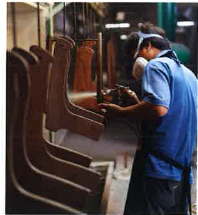
Spray-painting furniture with flammable varnish on an assembly line
