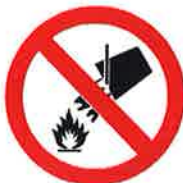
Do not extinguish with water
