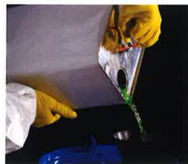
Dispensing solvent into a storage drum
