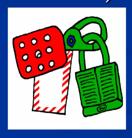
While repair or other work being performed on equipment must be locked out as defined by the Permit to work and Isolation Certificate
