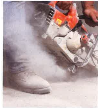
A petrol driven disc cutter is used to cut concrete. Vibration is delivered into both hands during use. Noise and dust will also be major health hazards
