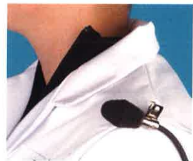
Recommended position for a dosimeter microphone Source: L108 Controlling noise at work (2nd ed.), HSE, 2005 ( www.hse.gov.uk/pubns/books/l108.htm )
