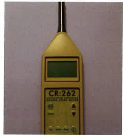
An Integrating Sound Level Meter (ISLM)
