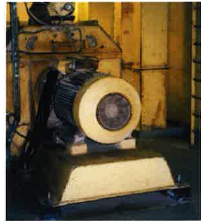
Anti-vibration mounts isolate grinder from supporting surface Source: L108 Controlling noise at work (2nd ed.), HSE, 2005 ( www.hse.gov.uk/pubns/books/l108.htm )
