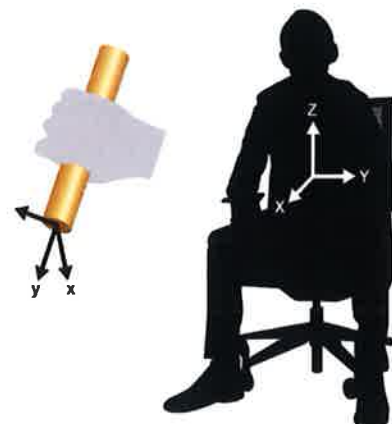
Axes of vibration for hand-transmitted and whole-body vibration
