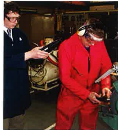
Making measurements with a hand-held sound level meter
