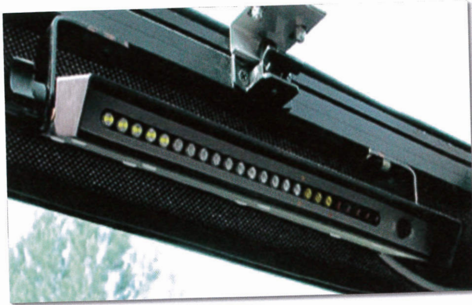
Cab Roof Located LMI Indicator
