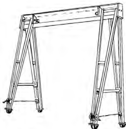
Figure 12.11 Self erecting gantry
