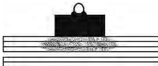
Figure 26.7 Magnetic lifters with variable power facilitates shedding of excess load
