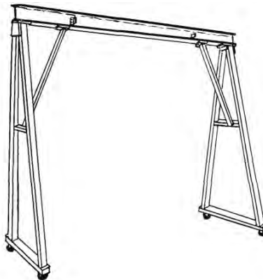
Figure 12.8 'A' frame gantry
