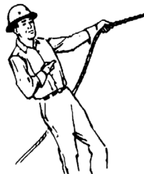
Fig. 20 RETRACT BOOM (Telescoping Boom) One Hand Signal . One fist in front of chest, thumb pointing outward and heel of fist tapping chest.
