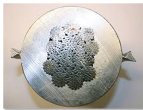
Cross- Section of a Pressed Ferrule Termination
