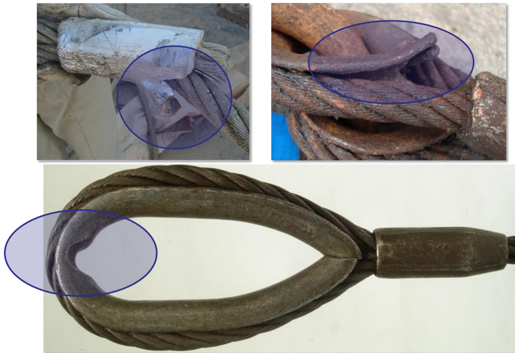
Damaged Reeving Thimble
