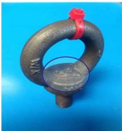
An eye nut with a threaded bar welded into it to make an eyebolt
