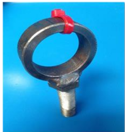
A bolt welded to a piece of steel pipe section to make an eyebolt
